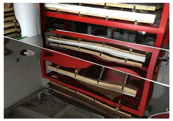
BA refers Bright Annealed. BA surface is a kind of bright treatment to the surface of ordinary stainless steel, which is white and bright, and its surface is highly reflective which can illuminate people's shadows. The mirror stainless steel plate is polished on the stainless steel surface with a polishing liquid through a polishing equipment, iron-red powder, nitric acid, and the surface formed by grinding with the wool felt makes the surface brightness as clear as a mirror.
