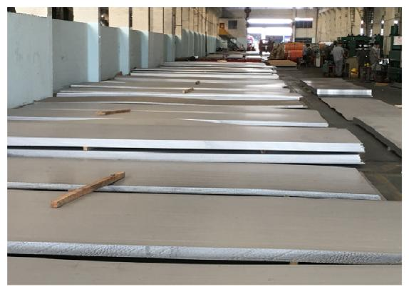
304L is a steel grade obtained by reducing the carbon content of 304 to less than 0.03%. Its general characteristics are almost the same as 304, but 304L stainless steel can inhibit the sensitization caused by the precipitation of chromium carbide between 500 and 900oC. , Improve the sensitivity of intergranular corrosion caused by welding, etc., so it is suitable for large-scale welding structure materials and pipe fittings that need to be used directly after welding.
